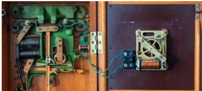
Top and above: dial and mechanism of a Gent's primary clock, which generates electrical impulses to control multiple secondary dial clocks.
